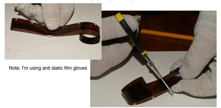
**2- Slide film into film holder:** Line up frame as shown in picture.
